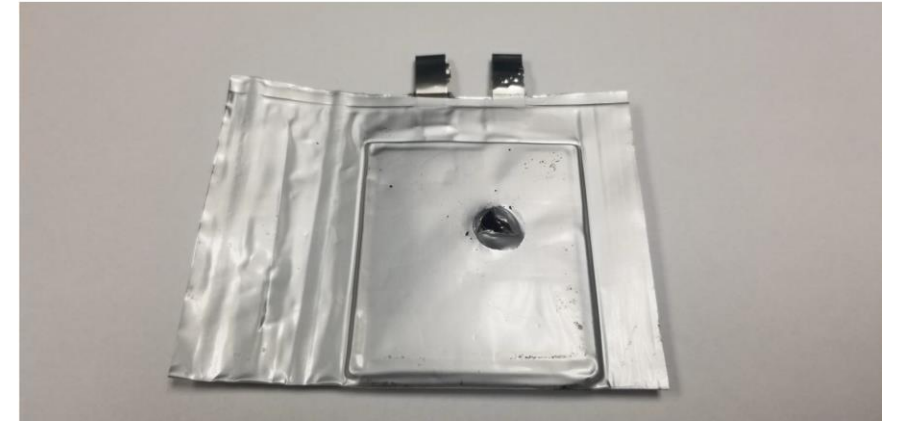
NPORE ® prevents thermal runaway in nail penetration test
